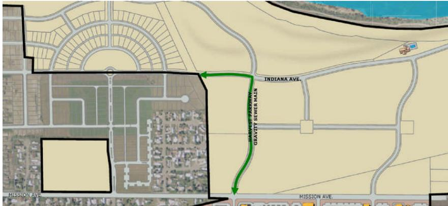
**Project Description:** Install sanitary sewer system improvements consisting of 2,200 lineal feet of gravity main and associated fittings and manholes.
