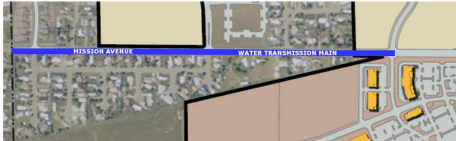
**Project Description:** Construct a water transmission main along Mission Avenue to Telido Station. Installation includes approximately 2,950 lineal feet of new water transmission main and associated fittings and valves.
